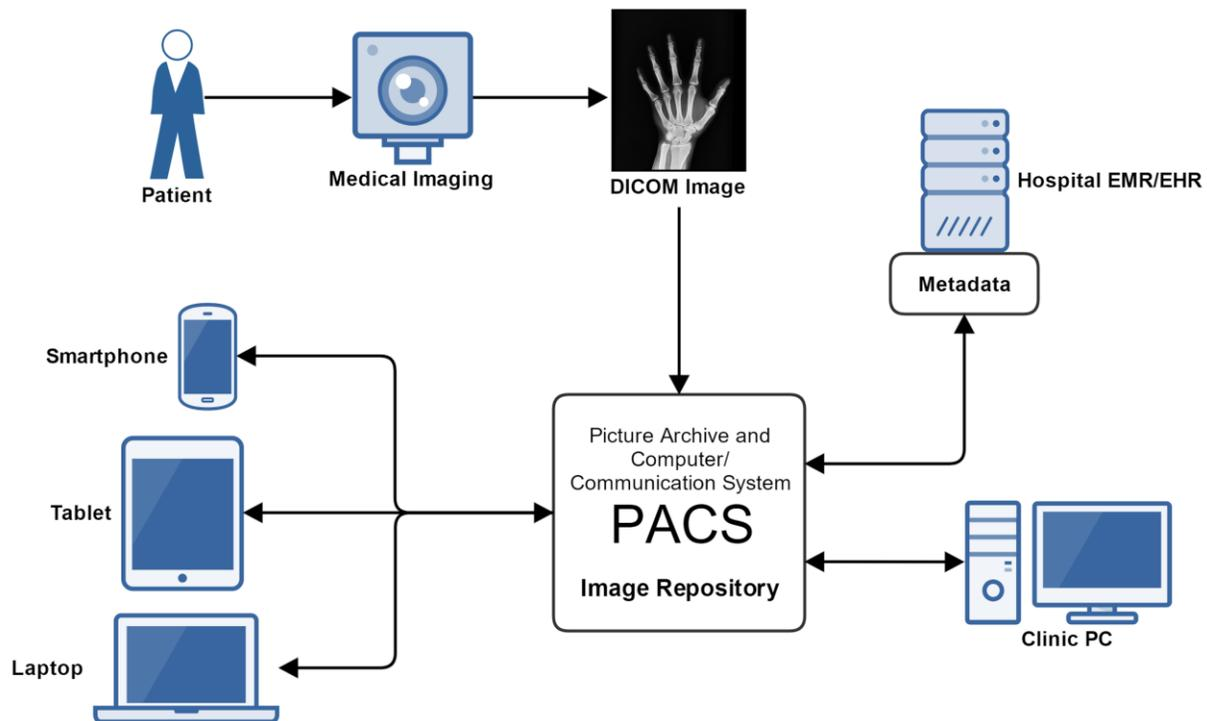
**Figure 2: Picture Archive and Computer/Communication System**
