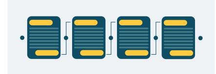
Transactons contain encrypted and digitally signed data along with an index that points to the prior block in the blockchain. Transactions are structured into blocks and recorded in chronological order.
