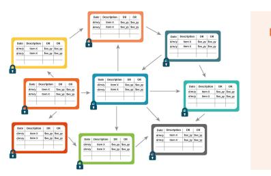
Blockchain is a decentralized P2P architecture. Members in the distributed network record digital transactions into a shared ledger. Each member stores an identical copy of the shared ledger and changes to the shared ledger are reflected in all copies.
